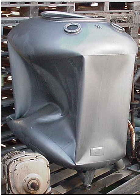
Picture: tank collapsed due internal underpressure. Although this time the explosion wasn't the reason, this can happen even to big industrial and agricultural silos
